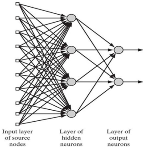
Figure 1. Multilayer feed forward network model [Haykin, 2005].
