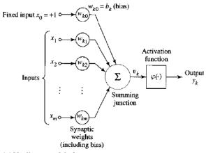
Figure 1.1 Nonlinear model of a neuron
