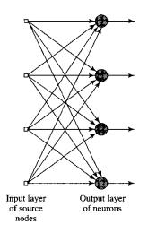
Figure.1.2 Feed-forward network with a single layer of neurons
