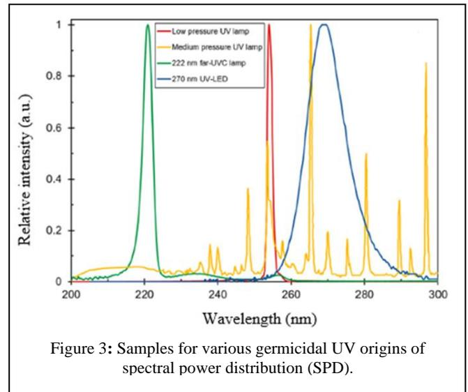
Figure 3: Samples for various germicidal UV origins of spectral power distribution (SPD).
